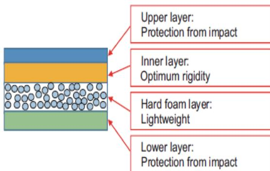
Fig. 2 Cross-section of the walls of the case. The case is lightweight, yet it provides strong protection.
