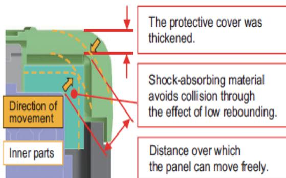
Fig. 1 Modified corner of the cassette. Breakage and internal damage to the cassette due to dropping can be avoided.
