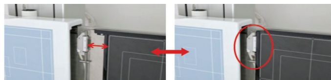
Fig. 3 The AeroDR 17"x17" radiographic stand has two functions. When a cassette is inserted, the cassette's lithium ion capacitor is automatically charged and wireless communication automatically changes over to wired communication.
