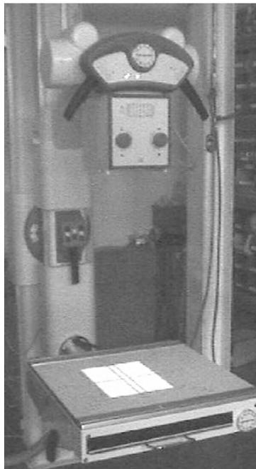
2. Position SID at 1 meter (use the SID scale of the Column).
