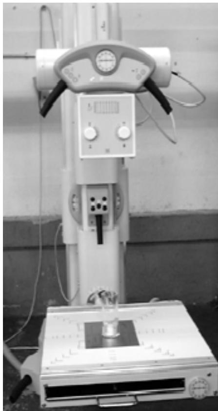
3. Turn on Collimator light and center the Collimator in relation to the Bucky Table-Top. Horizontal and transversal position of the light axes projected by the Collimator Lamp must be in line with the axes or film sizes marked on the Table-Top.
