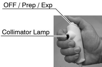
Radiographic exposures are controlled with the “*Prep*” (preparation) and “*Exp*” buttons on the X-ray Handswitch. The status of the exposure is shown by the “*Ready*” and “*X-ray On*” indicators for the duration of the exposure.
