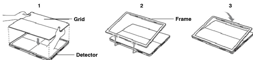
Check that the Grid is correctly mounted. A click sound means that the Grid is in place.
