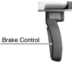
Both Tube-Collimator Assembly Handgrips have a Brake Control that releases or locks Column rotation and vertical and telescopic Arm movements. This control also releases the Arm Catch when in parking position.
