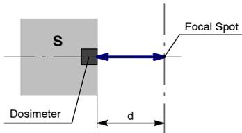
**d** = DISTANCE FROM THE AXIS OF THE X-RAY BEAM TO THE DOSIMETER
