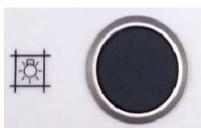
This button is used to turn ON the Collimator Lamp from the Control Panel.
